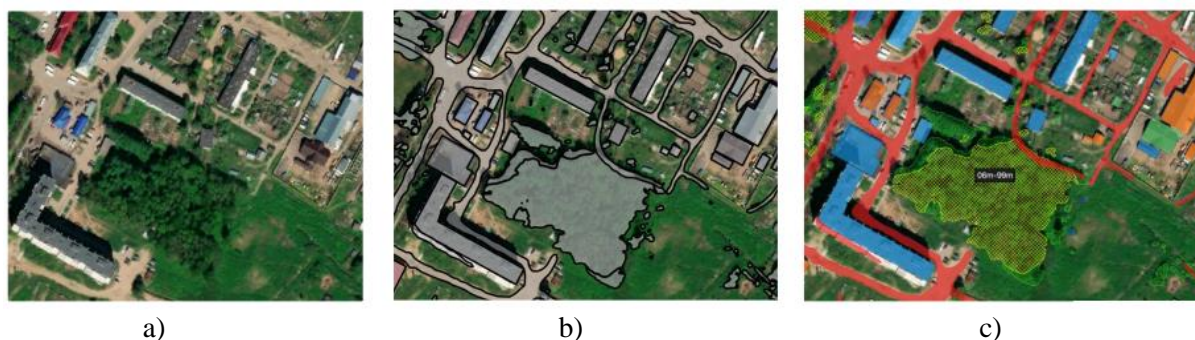
Figure 1 – a) Satellite image before neural network processing; b) Recognition of objects by satellite pictures (outlines); c) Adding some additional semantic attributes to each object
