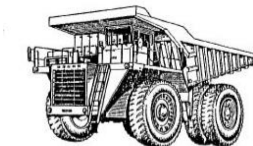
Figure 2 Dump truck BelAZ - 75211 with a carrying capacity of 180 tons.
