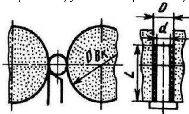
$$T_o = \frac{L}{n_d \cdot S_{\text{рад}}} \cdot K; \quad n_d = \frac{n_{\text{BK}} \cdot D_{\text{BK}}}{D}; \quad L = a = \frac{D - d}{2},$$
